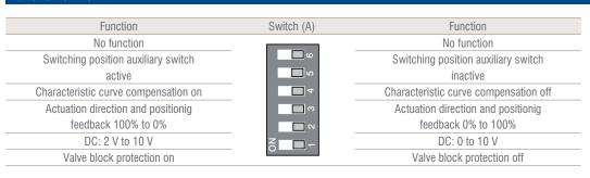
The valve functions are adjusted with switch A by placing the dip switches 1 to 6 in the desired position. The switch is located under the wiring connection cover.
