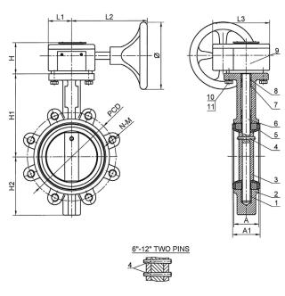
Drawing details representative of DN 200 to DN 300 valve construction. For details of valve construction for sizes DN350 to DN 600 please contact your local Conex Bänninger representative.
